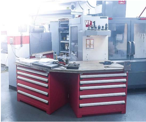
The newest addition to Rotuba’s machine shop is a Haas VF1 CNC machine to make intricate gages for quality control.
